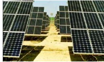
“...two types of Siemens PV modules—single-crystalline silicon and thin film copper indium diselenide. ... Over their lifetime, **these solar panels generate 9 to 17 times the energy required to produce them.**”
